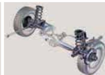
The heavy-duty coil spring suspension, incorporating telescopic shock absorbers and a torsion bar, provides confident handling.
